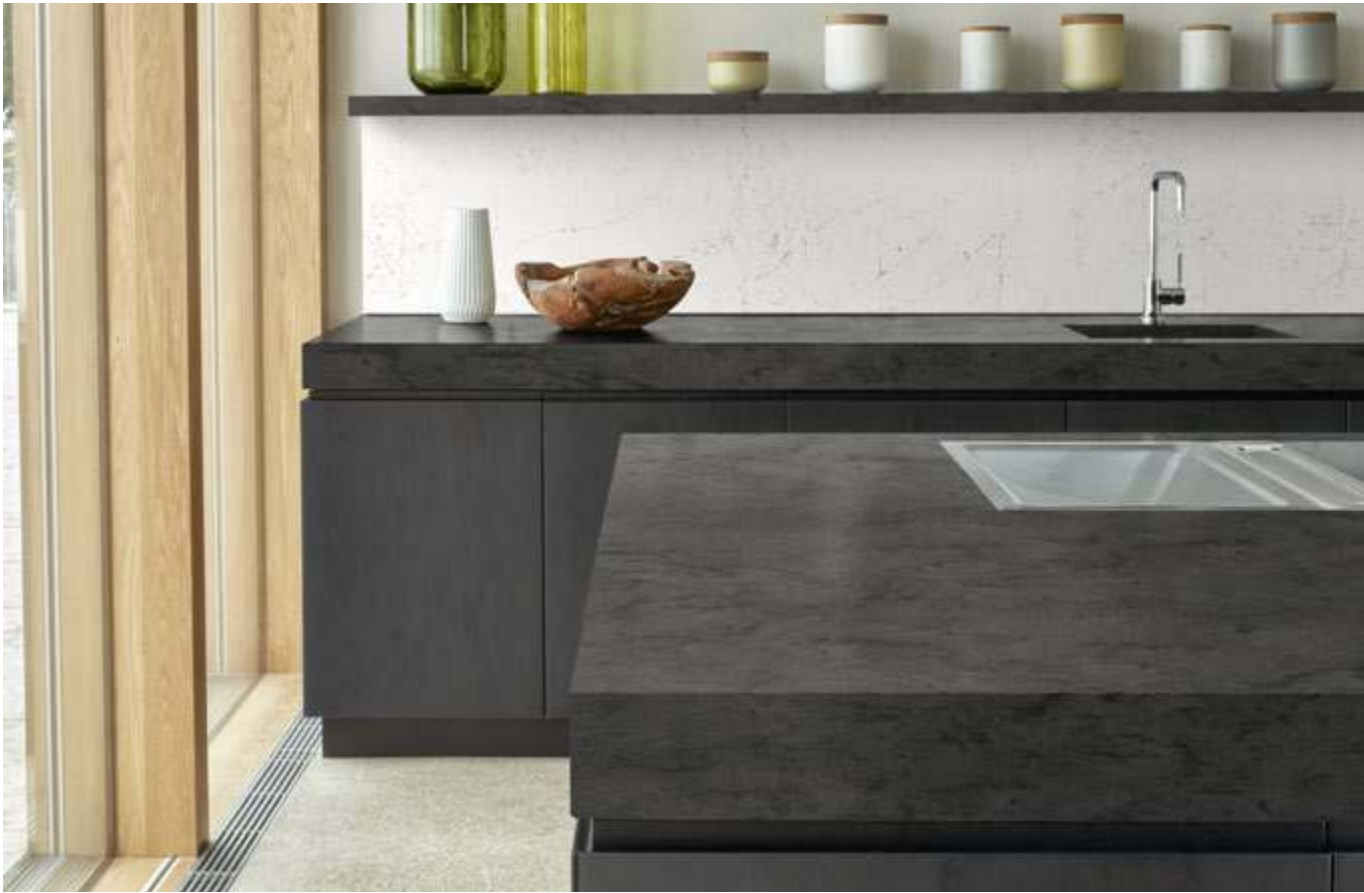
Two-toned kitchen interior with custom-designed Corian® sink, backsplash in Corian® Quartz (Bianco Marmor color); countertops in Corian® Solid Surface (Carbon Aggregate color) with side panels in Corian® Solid Surface (Carbon Concrete color).
